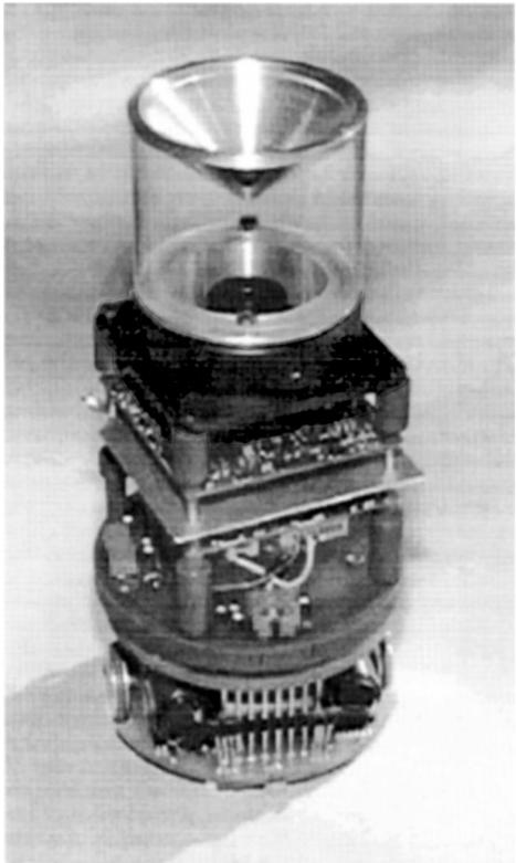
*Figure 2.* Khepera™ robot with camera module and custom made conical mirror, which permits sampling of the environment over  $360^\circ$ , in a range of  $\pm 10^\circ$  about the horizon.
