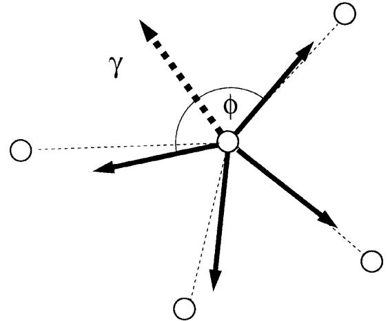
Figure 6. The robot estimates the directions to all connected vertices (black arrows). The largest open angle is denoted by  $\Phi$ . The next exploration step will be directed along  $\gamma$  into the middle of  $\Phi$ .
