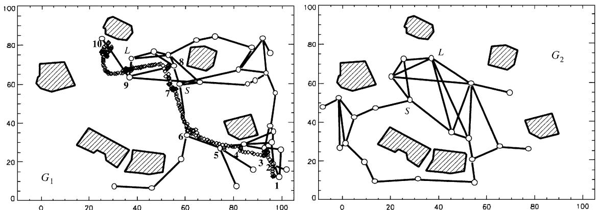
Figure 12. Two view graphs recorded by the Khepera robot with different start positions  $S$ . Circles denote locations of snapshots, lines recorded edges between them. The sample trajectory (diamonds) in  $G_1$  started at vertex 1. Vertex  $L$  is a possible linking place between  $G_1$  and  $G_2$  (see discussion).
