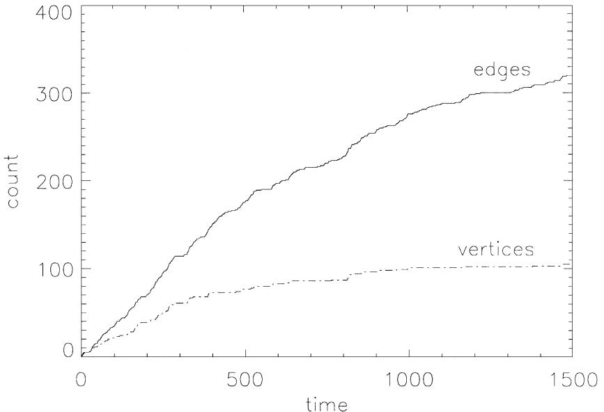
Figure 11. Number of graph vertices and edges as a function of exploration time during a simulated exploration. The number of edges continues increasing when the number of vertices has saturated.
