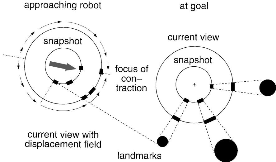
Figure 5. A robot with omnidirectional sensor uses a snapshot taken during a previous visit to find back to the goal position. After moving away from the goal, the images of the surrounding landmarks are displaced to new image positions, as denoted by the arrows at the current view. If the robot moves such that it reduces the displacements it will finally find back to the goal (after Cartwright and Collett, 1983).
